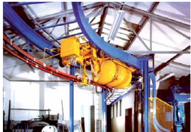
Feed and control of a concrete skipper
